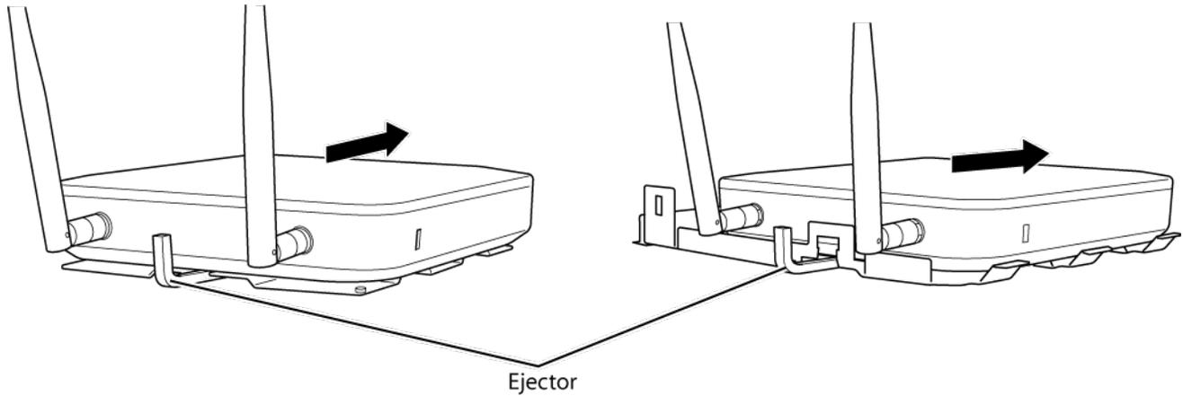
Insert the ejector key to raise the locking clips, then gently slide the AirStation off in the direction shown.
