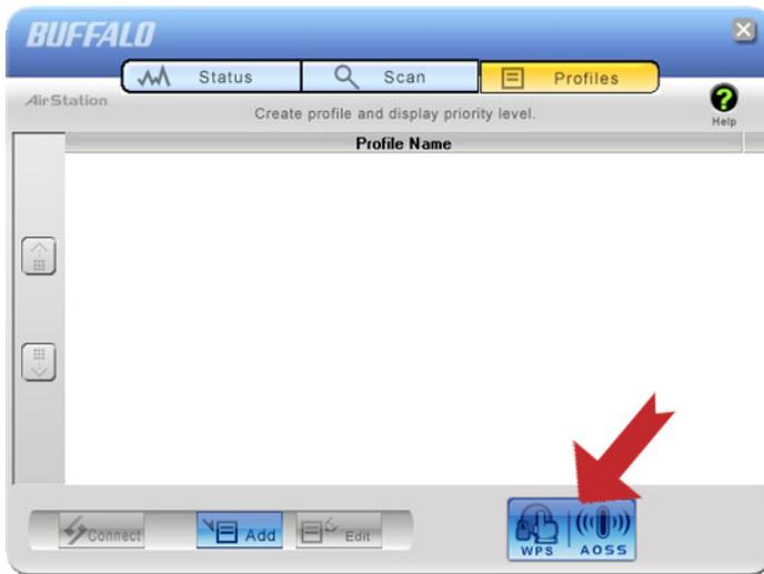
It will take several seconds for your wireless connection to be configured. When the 2.4 GHz and 5 GHz LEDs on the front of the AirStation stop flashing and glow steadily, the connection is complete.
