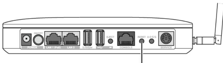
To return the AirStation to factory default settings while it is powered on, press and hold the reset button for 3 seconds.
