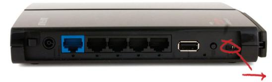
The second AirStation will be configured as a repeater/bridge. Make sure that its switch is set to "OFF" (the middle position). Use a RJ-45 Cat5 Ethernet cable to connect LAN ports of the two AirStations. Power up the second AirStation. Connect a PC's Ethernet port to another RJ-45 port on the main router (the first AirStation). You will use this PC to configure the settings of the AirStations.
