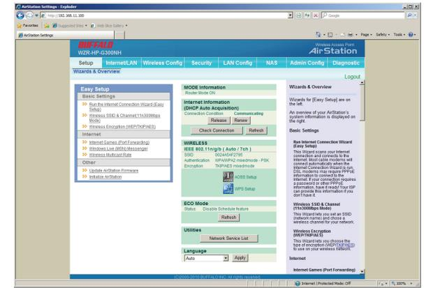
Once the bridge is working, you may enable encryption to limit who may use it. To configure encryption for the router AirStation, open its configuration utility (192.168.11.1) and navigate to *Wireless Config - Basic (n/g/b)*. Select the desired values for *Wireless Authentication* and *Wireless Encryption*. Enter a passphrase for the network in the *WPA-PSK* field. Passphrases may be 8 - 63 characters long and should contain both numbers and letters.
