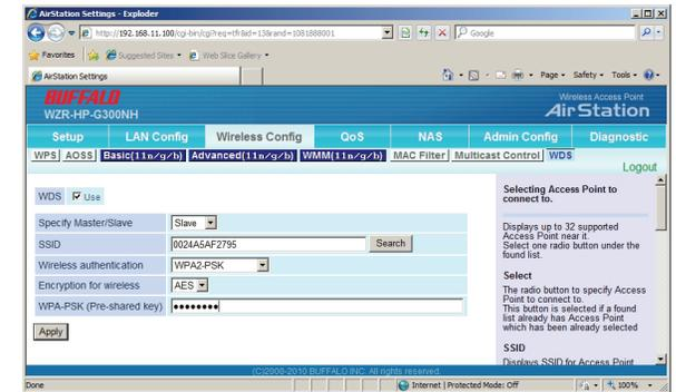
To configure encryption for the bridge AirStation, open its configuration utility (192.168.11.100) and navigate to *Wireless Config - WDS*. Select your desired *Wireless Authentication* and *Wireless Encryption*. Enter the passphrase in the *WPA-PSK* field. It should be the same as the router's.
