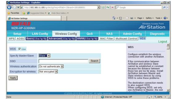
Find your router AirStation's SSID on the list and select it. Click *Select*. Click *Apply* to configure the bridge. The AirStation will restart.
