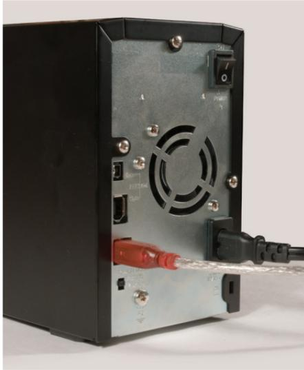
Connect the USB or firewire cable to your Mac or other device you are adding the DriveStation to.
