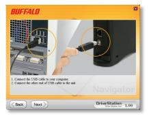
The wizard will guide you through installation. First, you'll install the DriveStation FlexNet as a USB device. Then, you'll switch modes and install the DriveStation FlexNet in LAN mode as a NAS device. Follow the directions on each screen and continue pressing *Next* to step through the installation.
