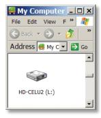
In USB mode, the DriveStation functions as a normal external USB hard drive. It can be accessed from My Computer. By default, it will receive the next available drive letter and will be named *HD-CELU2*.
