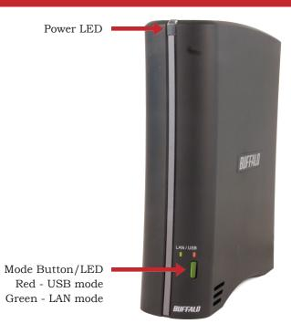
Note: The DriveStation FlexNet can be connected to a computer as both an Ethernet NAS and a USB external hard drive at the same time. To switch between the two modes, hold down the mode button for a few seconds and then release it.
