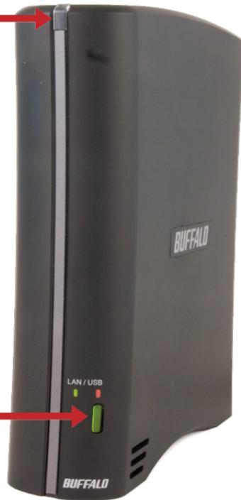
Note: The DriveStation FlexNet can be connected to a computer as both an Ethernet NAS and a USB external hard drive at the same time. To switch between the two modes, press the mode button.
