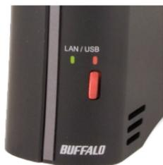
In USB mode, the mode button will glow red. If it's green, press it. The LED will change to red. To use the DriveStation in USB mode, it must be connected to your computer with a USB cable.
