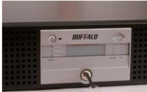
Pull on the right hand side of the front panel to remove it.
