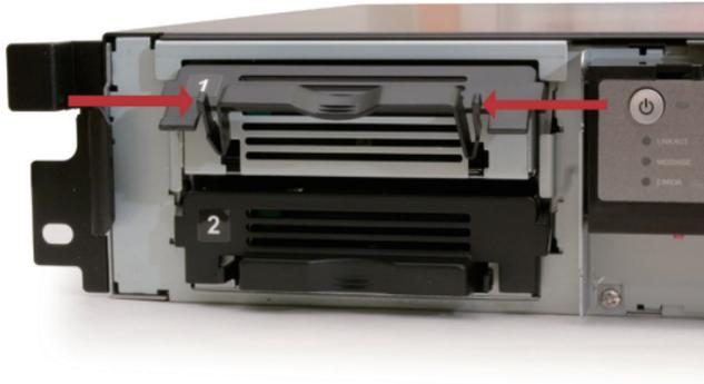
Squeeze the tabs gently and swing the tray latch upward.
