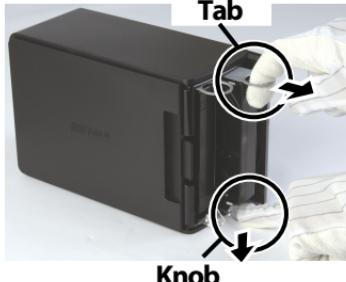
Press the release below the drive and pull the tab above the drive out 2 cm (about 1 inch) .
