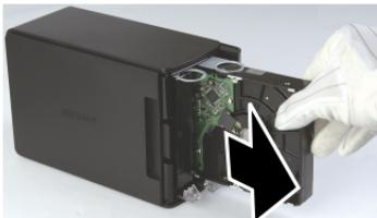
Remove the failed drive.
