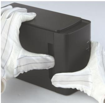
Pull the front cover forward while pressing gently on the hollow on the left side.
