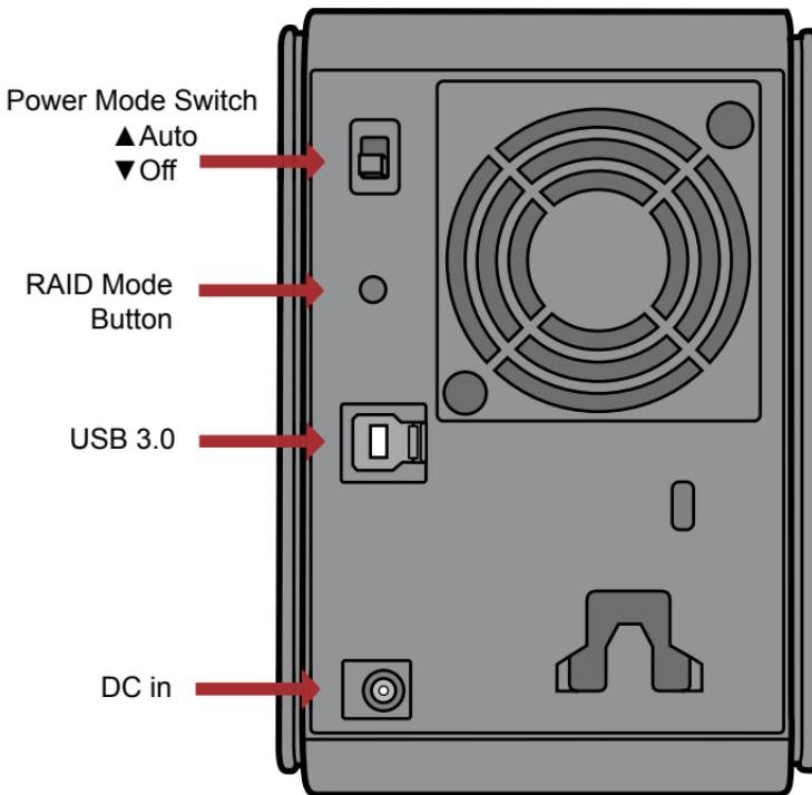
Note: To change between RAID modes, you may use either the RAID utility or the RAID mode button. The RAID utility is included with the software on your DriveNavigator CD. For more information on using the RAID mode button, see the Reference Guide.
