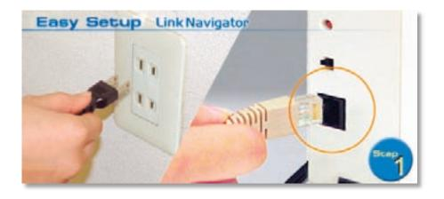
Plug the LinkStation's power cord into the back of LinkStation. Then, plug the other end of the power cord into a power outlet.
