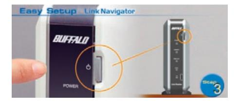
Turn the LinkStation on by pressing the power button until the green Power LED begins to flash.
