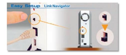
On the rear of the LinkStation, flip the black *Cable Selection* switch. This switch tells LinkStation whether to communicate over a Crossover or Patch cable. Verify that the LINK/ACT LED on the front of LinkStation is lit (see *page 9*'s picture). If it is lit, continue to *page 12* to continue setting up LinkStation. If the LINK/ACT LED is still not lit, try moving the switch to the other position. If that doesn't help, turn to the next page to check for common problems.
