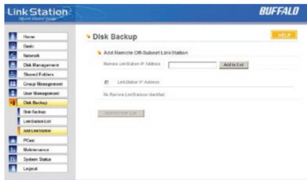
To add a remote LinkStation to your network, enter its numerical IP Address in the *Remote LinkStation IP Address* field and click the *Add to List* button. For remote LinkStation backups, make sure both firewalls are configured to allow traffic in and out of their networks.
