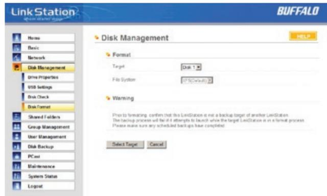
To format a hard drive or array, select it from the *Target Disk* drop box. Choose the file system desired from the *File System* dropdown (internal drives can only be formatted with XFS). Note that FAT32 has a 4 gigabyte filesize limit for individual files. If you choose FAT32 for your file system, you will not be able to store single files larger than 4 gigabytes on the drive. Use of the *XFS* or *EXT3* file systems is recommended. Press *Select Target Disk* when done, and then *Start format*.
