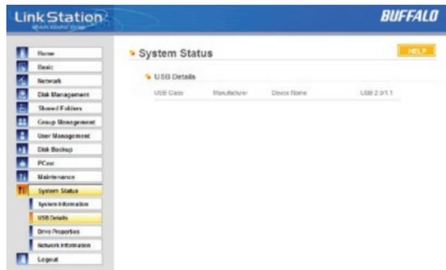
This page shows you details on USB hard drives and UPSs plugged into your LinkStation. In this example, no USB hard drives are plugged in to the LinkStation.
