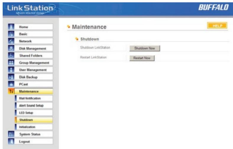
From the *Shutdown* page, press *Apply* to shutdown LinkStation. This has the same function as holding down the power button on the front of LinkStation, but may be done remotely. Turning on the LinkStation after a shutdown requires a physical button push on the front of LinkStation. The *Restart Now* button simply reboots the LinkStation, bringing it back to functionality after about 120 seconds.
