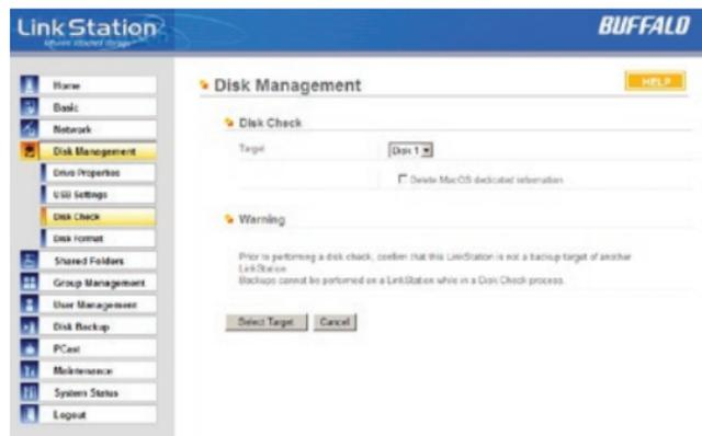
Disk check checks any of your hard drives for errors. To use disk check, select the disk that you want to check from the target pulldown and click *Select Target*. Then click on *Start Disk Check*.
