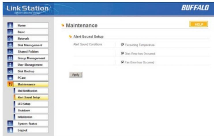
Alerts can be configured on the LinkStation to make audible noises when a problem is detected. Along with the audible noise, alert emails will be sent out if *Mail Notification* was properly configured. Please select the features you would like to receive an audible sound alert from and then press the *Apply* button.
