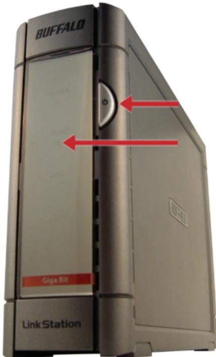
Press the *power button* on the front panel. LEDs will blink as your LinkStation boots up.
