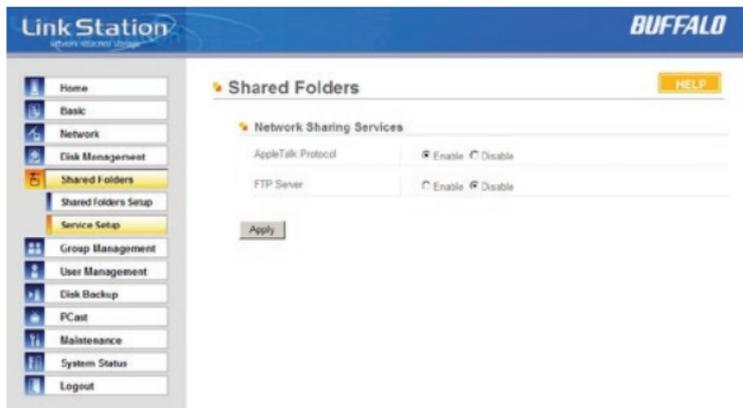
To allow FTP Access to LinkStation, choose *Enable* for *FTP Server*. To enable legacy AppleTalk support, choose *Enable* for *AppleTalk Protocol*.
