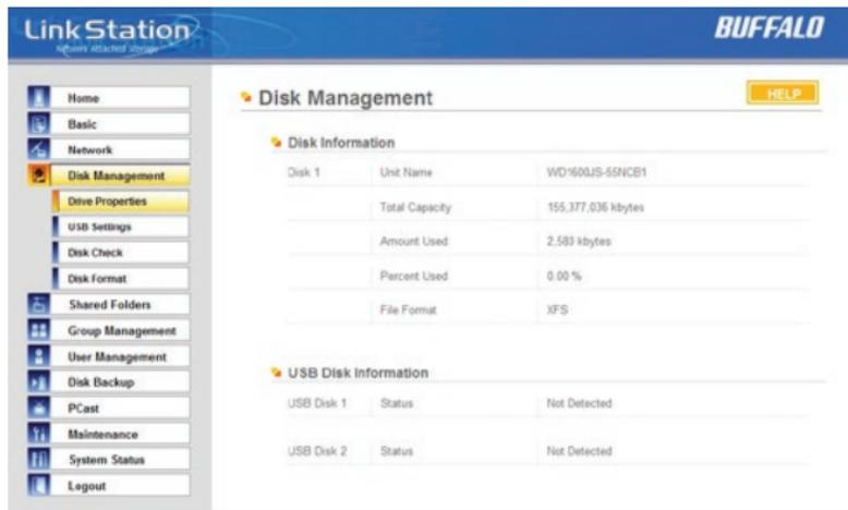
The screenshot displays the LinkStation web interface for Disk Management. The left sidebar contains navigation options: Home, Basic, Network, Disk Management (selected), Drive Properties, USB Settings, Disk Check, Disk Format, Shared Folders, Group Management, User Management, Disk Backup, PCast, Maintenance, System Status, and Logout. The main content area is titled 'Disk Management' and includes a 'HELP' button. It is divided into two sections: 'Disk Information' and 'USB Disk Information'.
