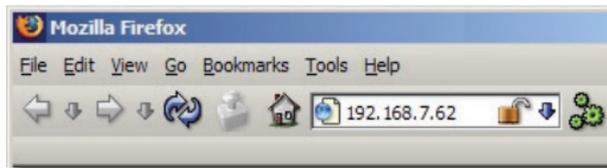
The Configuration GUI may be accessed at any time by typing the IP address of your LinkStation into the URL bar of a browser running on a computer connected to the same network as the LinkStation. This works perfectly with OS X, Linux, and other non-Windows PCs.
