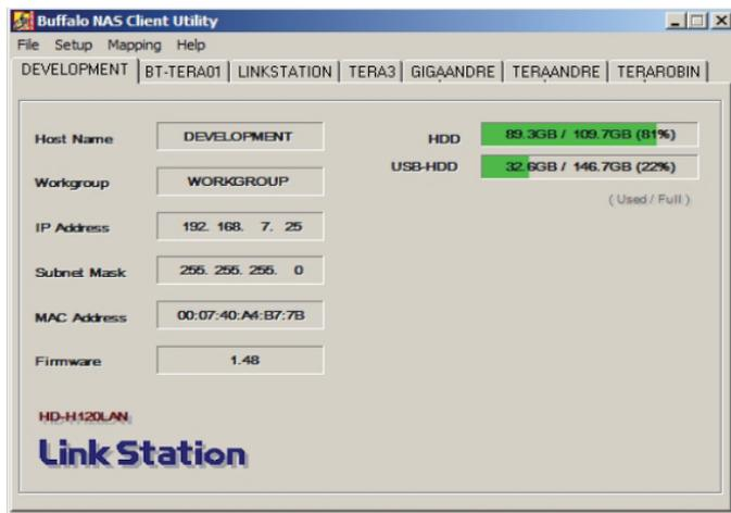
This is the *Buffalo NAS Client Utility*. Installed on your PC, it allows you to access each of the LinkStations (and TeraStations) on your network. Click *Refresh List* to get tabs for each of your LinkStations. Each tab shows the Host Name, Workgroup, IP Address, and Subnet Mask of the associated LinkStation, as well as the version of firmware it's running.
