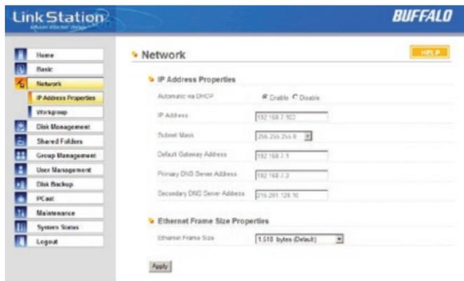
In most networks, LinkStation will get its IP Address automatically from a DHCP server. You may disable DHCP here. If DHCP is disabled and an IP Address is not set manually, it will default to *192.168.xxx.xxx* with subnet mask 255.255.0.0. The LinkStation's *IP Address, Subnet Mask, Default Gateway Address, and DNS Server address* may all be entered manually under *IP Address Properties*.
