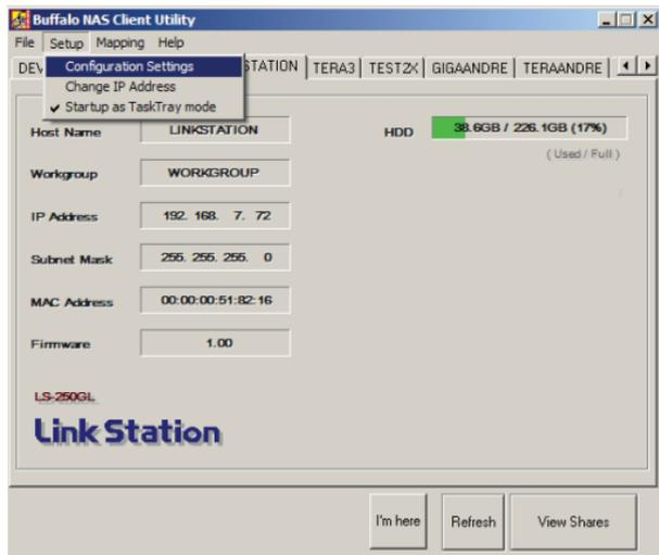
You may also open the Configuration GUI from NAS Navigator by clicking on *Setup* and choosing *Configuration Settings*.
