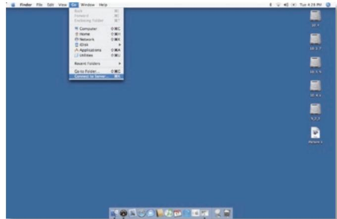
In the *Server Address* field, enter your LinkStation's IP address in the form *smb://ipaddress* (where "ipaddress" is your LinkStation's IP address), and click *Connect*.
