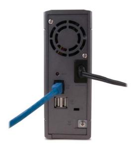
Connect the power plug to a surge protector or power outlet. Plug the other end of the Ethernet cable into a hub, switch, or router on your local network.
