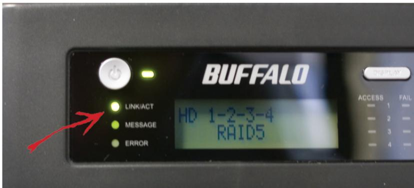
If the LINK/ACT LED on the front of TeraStation is **not** lit, your TeraStation is not properly connected to your network. Make sure that:
