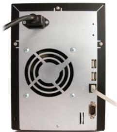
Connect the power plug to a power outlet. Plug the other end of the Ethernet cable into a hub, switch, or router on the network.
