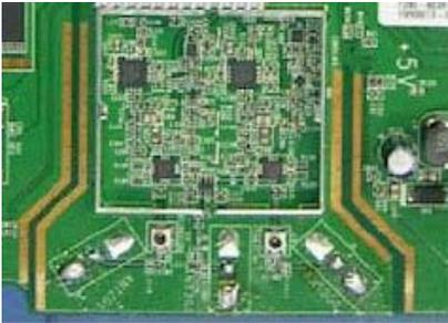
**Non-adjustable internal PCB antennas**
