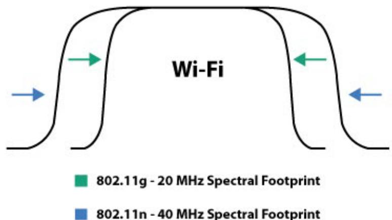
**802.11n Performance (MIMO 2x2, 3x3, etc):** MIMO allows for multiple antenna paths to be used to combine multiple signals for increased range and performance. The amount of antenna paths per device can be complicated to understand, but it has serious implications for performance. Many Wi-Fi equipment manufacturers choose to use terminology like 2x2 (two-by-two) to indicate what MIMO technology is in the product.
