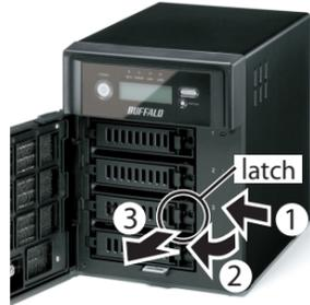
**10** Once the lock has swung out 45°, slide the drive cartridge out.
