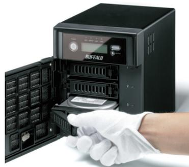
**11** Insert the replacement drive with the lock open.
