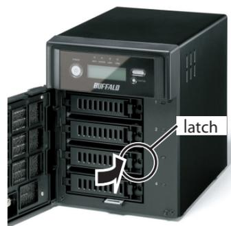
**13** Close the front cover. If the TeraStation was off, press the power button to turn it on.
