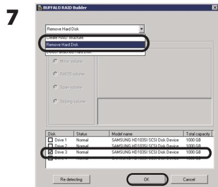
Select [Remove Hard Disk] from the dropdown menu. Select the hard disk to remove\* and click [OK].
