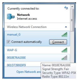
Select the target AirStation's name and click [Connect]. If you will be connecting to this device in the future, checking [Connect automatically] is recommended.
