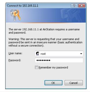
When this screen appears, enter [root] (in lower case) for the user name and the password that you set during initial setup. Click [OK].
